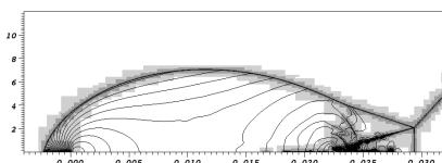
Cartesian base grid  $360 \times 160$  cells on domain of  $36 \text{ mm} \times 16 \text{ mm}$  with up to 3 refinement levels with  $r_f = 2, 4, 4$  and  $\Delta x_{1,2} = 3.125 \mu\text{m}$ , 38 h CPU
