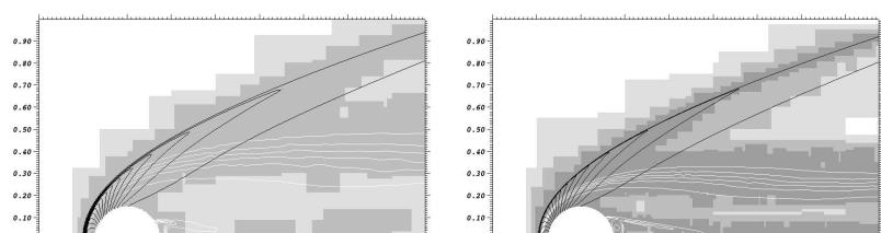
Iso-contours of  $p$  (black) and  $Y_{\text{H}_2}$  (white) on refinement domains for 3-level (left) and 4-level computation (right)
