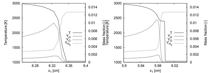
Approximation of H<sub>2</sub> : O<sub>2</sub> detonation at  $\sim 1.5 \text{ Pts}/l_{ig}$  (left) and  $\sim 24 \text{ Pts}/l_{ig}$  (right)
