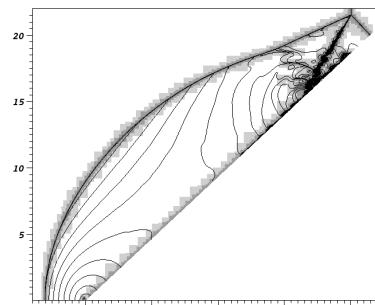
GFM base grid  $390 \times 330$  cells on domain of  $26 \text{ mm} \times 22 \text{ mm}$  with up to 3 refinement levels with  $r_f = 2, 4, 4$  and  $\Delta x_{e,1,2} = 2.849 \mu\text{m}$ , 200 h CPU
