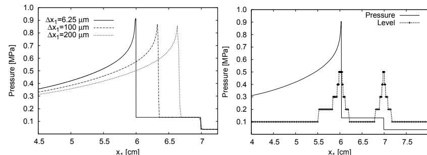
Left: Comparison of pressure distribution  $t = 170 \mu\text{s}$  after shock reflection. Right:
