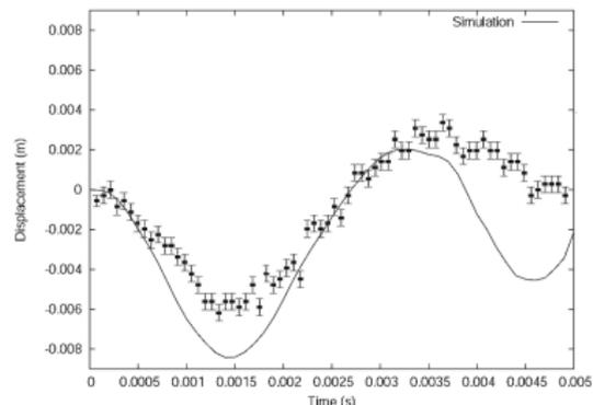
Tip displacement in simulation and experiment
